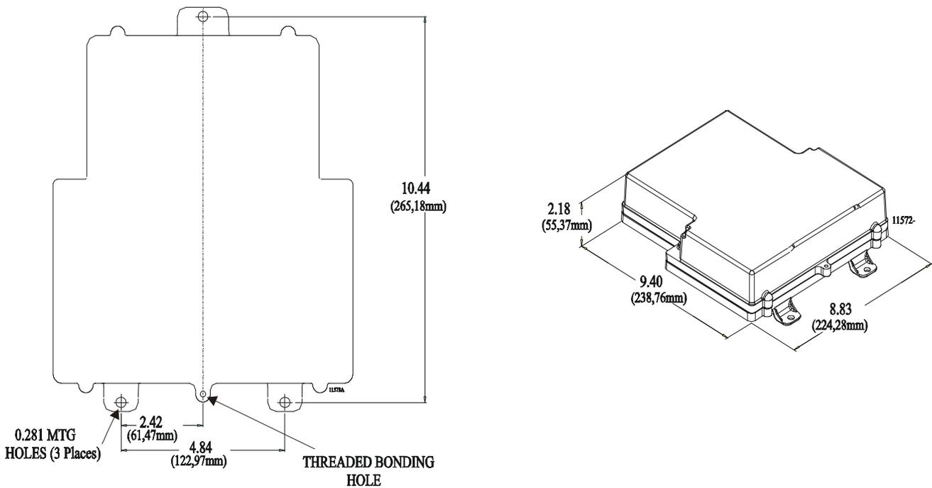
**Figure MMC-343-4: Station Expander Dimensions**
