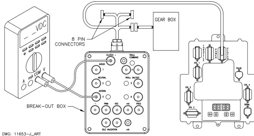
**Figure MM13927-11: Clutch Connections Astern Solenoid**
