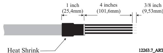
**Figure 4-16: Clutch Hard-Wired Cable**
