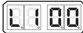
**Figure 5-35: Display LED L1 - Solenoid**
