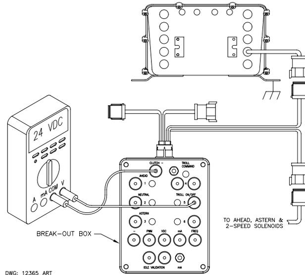
**Figure MM13927-14: 2-Speed Connections**
