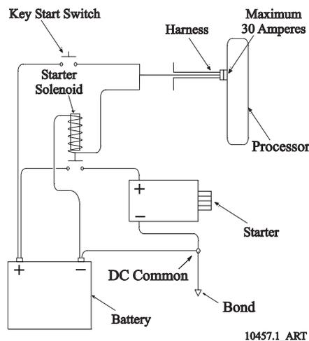
Figure 4-2: Start Interlock Connections
