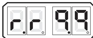
**Figure 10-8: Example Display Software Revision Level View**
