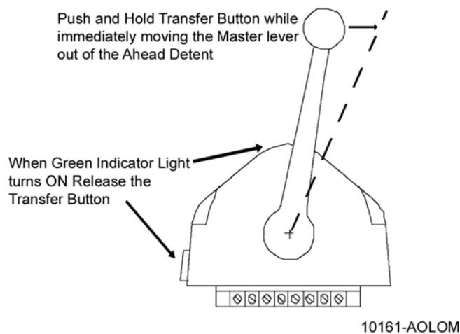
**Figure 2-9: One Lever Operation Mode**
