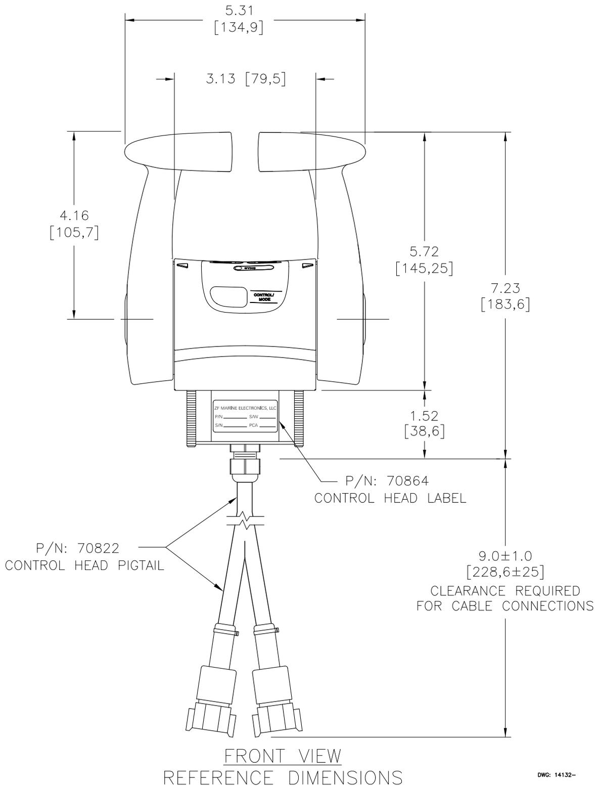
Figure MMC-337-5: 4200 Control Head - Front View Dwg #14132
