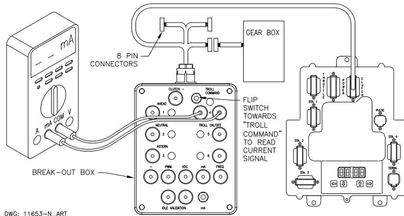
**Figure MM13927-13: Troll Connections (Proportional Solenoid)**
