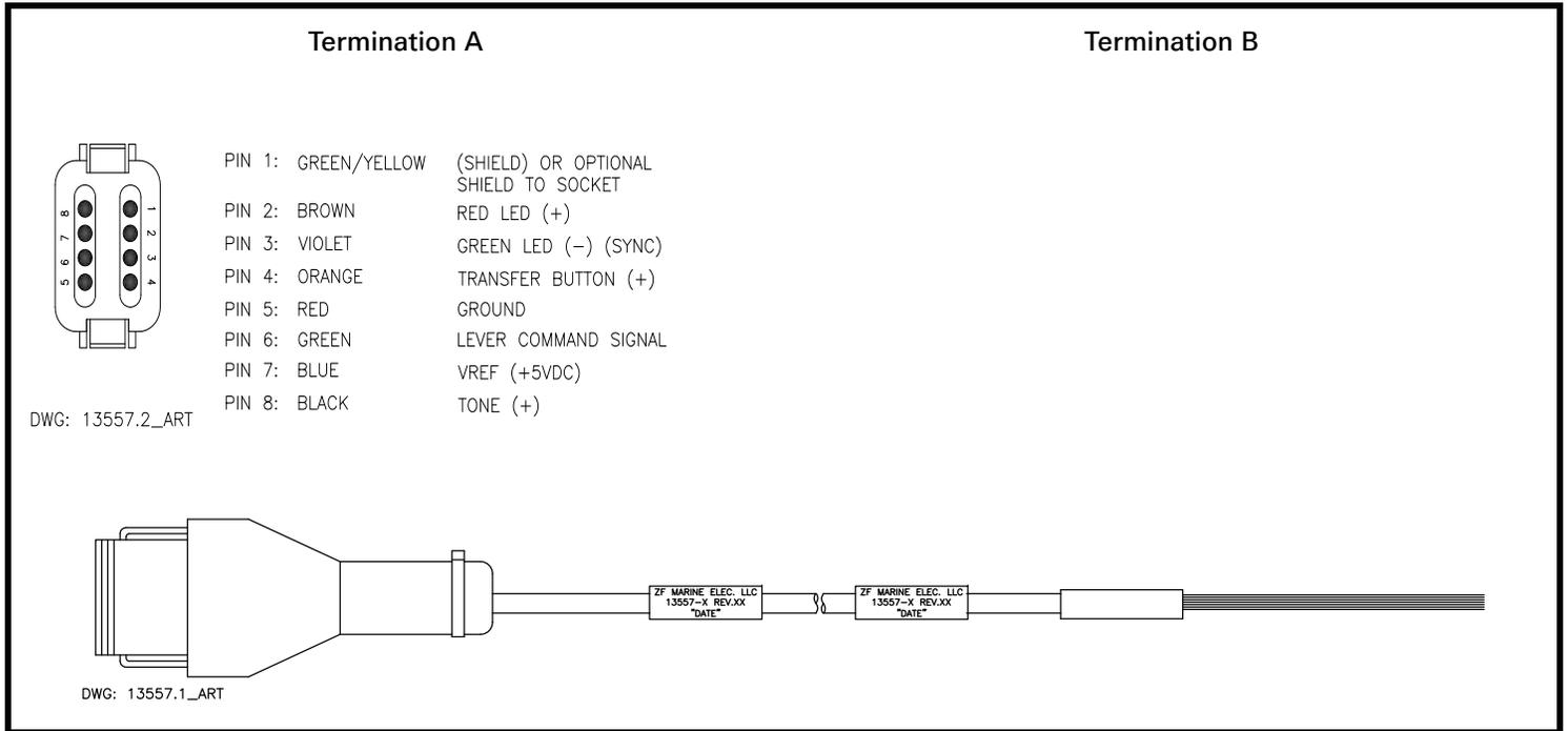
Table 10-62: Wire Harness - Control Head Two Connectors (p/n 14261-XX)
