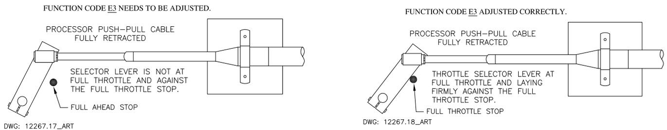
Figure 5-4: Throttle Push-Pull Cable Full Throttle Position
