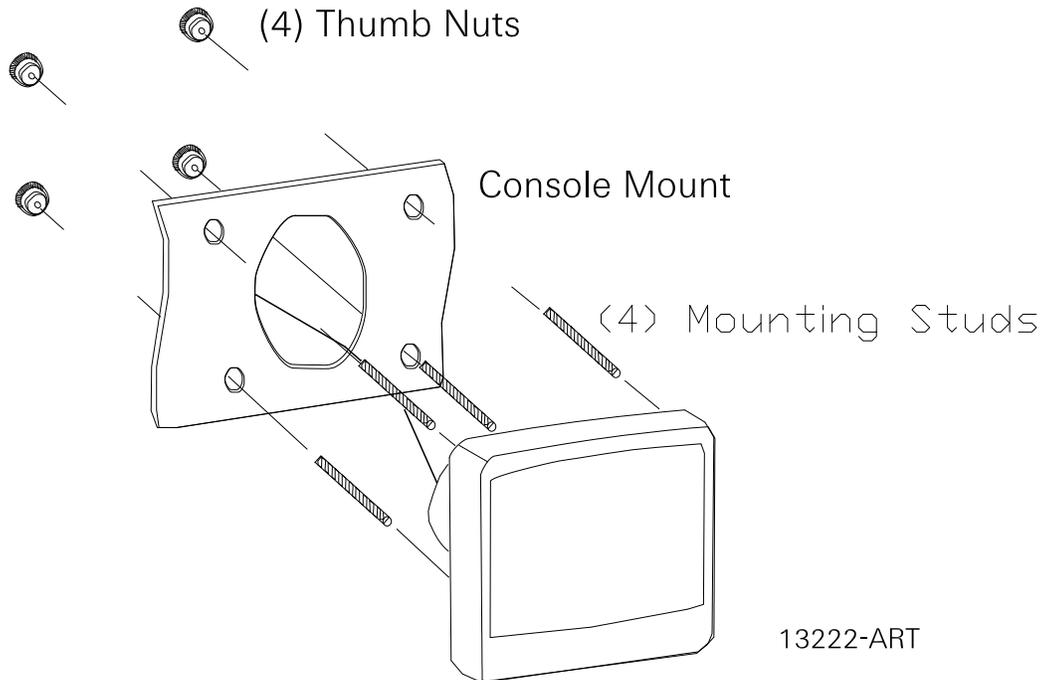
**Figure MM70179-13: On Console Mounting**
