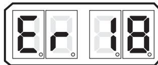
Figure 5-6: Display LED Error Menu Example
