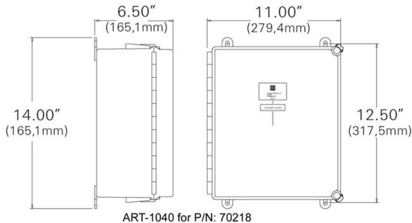
**Figure 3-2: Enclosure (P/N 70218) Dimensions**
