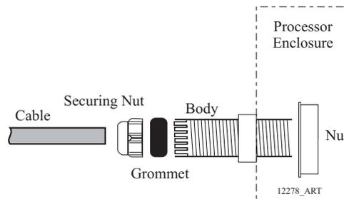
Figure 4-4: Liquid Tight (Watertight) Connector Installation
