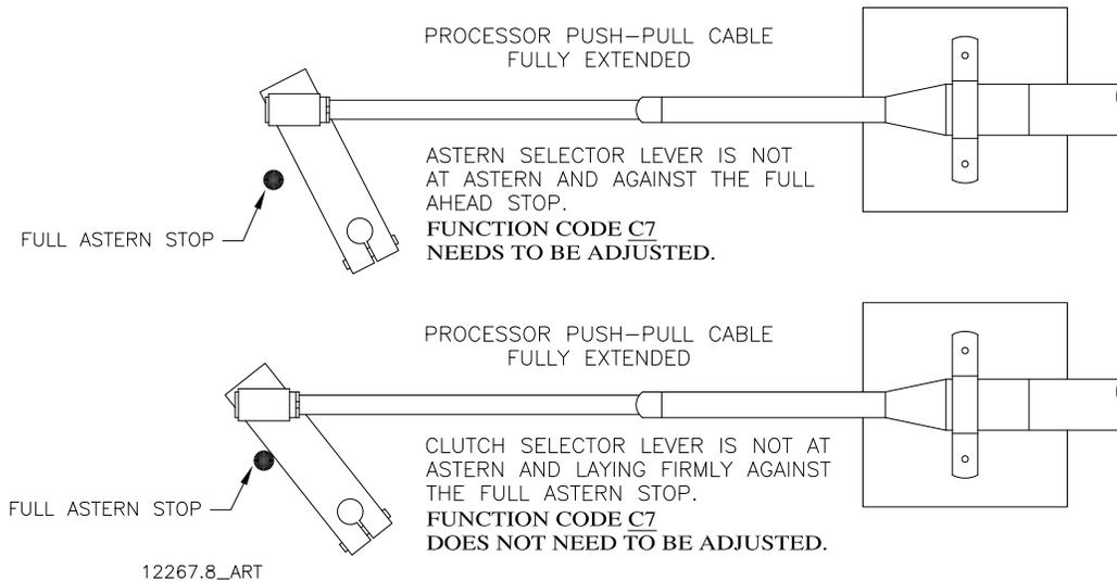
**Figure 5-27: Clutch Push-Pull Cable Astern Position**
