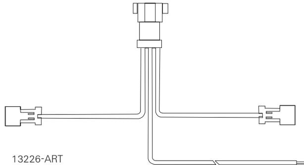
**Figure MM70179-16: Wire Harness (70186), Multi-drop**
