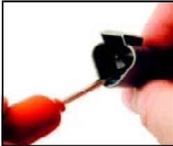
2. To remove the contacts, gently pull wire backwards, while at the same time releasing the locking finger by moving it away from the contact with a screwdriver.
