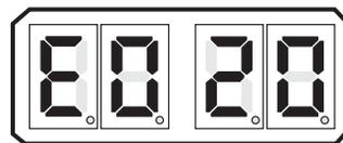
**Figure 5-17: Display LED E0 - Servo**
