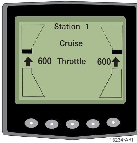
Figure MM70179-5: Ahead Detent
