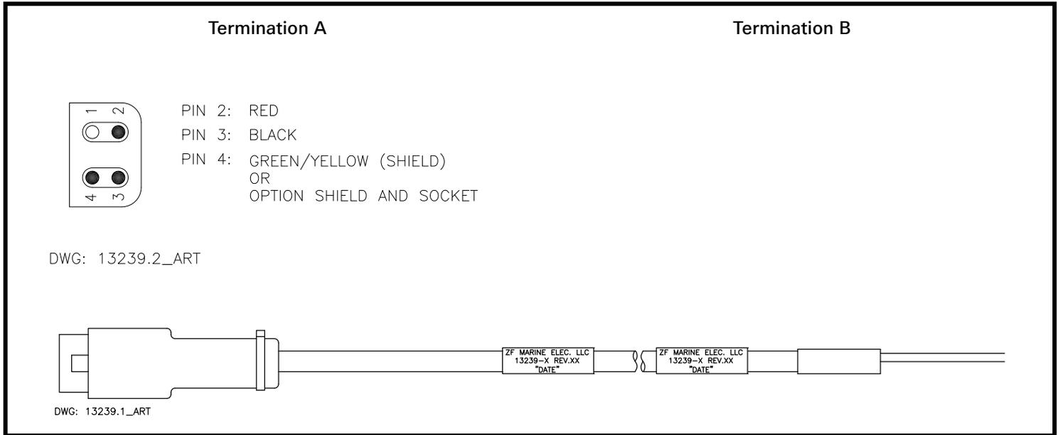
Table 10-64: Wire Harness- Tach Sensor with 3 pin plug (p/n 13334-XX)
