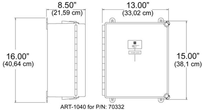
**Figure 3-3: Enclosure (P/N 70332) Dimensions**
