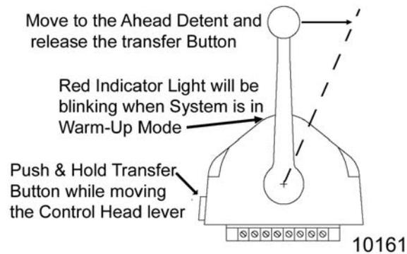
**Figure 2-5: Control Head Warm-Up Mode**
