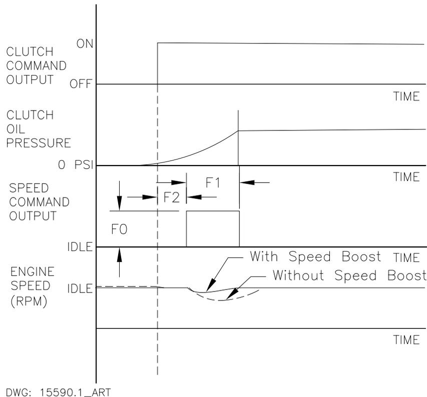
Figure 8-6: Speed Boost Usage Graph
