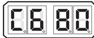
**Figure 5-26: Display LED C6 -Servo**
