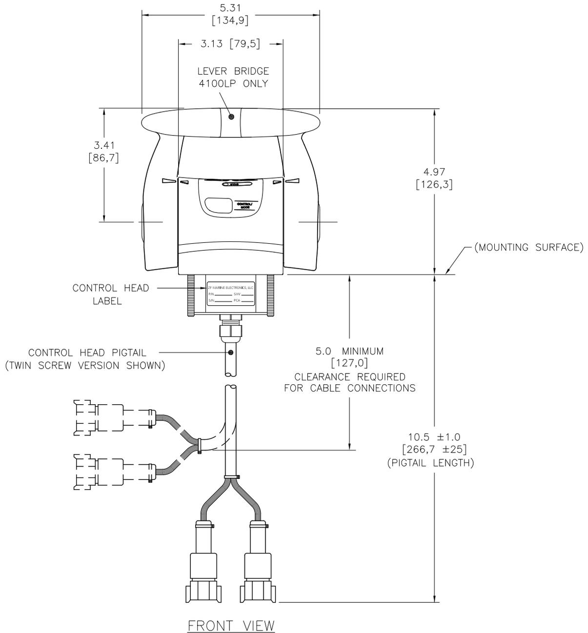
Figure MMC-337-7: 4100LP Control Head – Front View Dwg #13932ART-8
