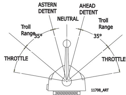
**Figure 5-30: Control Head 20 Degree Troll Range - Type 1**     **Figure 5-31: Control Head 35 Degree Troll Range - Type 2**
