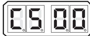
Figure 5-29: Display LED C5 - Solenoid
