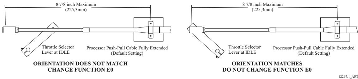
**Figure 4-23: Throttle Push-Pull Idle Orientation to Selector Lever**
