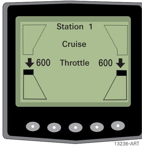
Figure MM70179-7: Astern Detent - Idle Throttle
