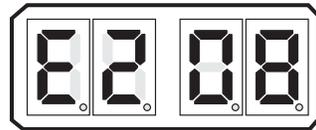
Figure 6-8: Display LED E2 - Electronic
