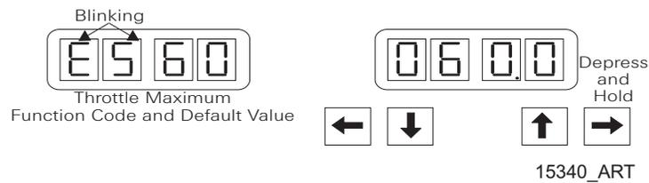
**Figure MMC-343-9: Display LED Four Digit Value**
