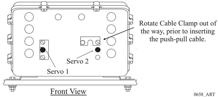
**Figure 4-21: Processor Cable Clamp Rotation**
