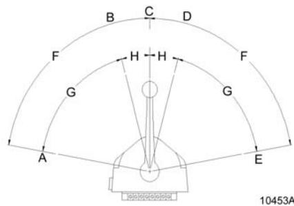
Figure 2-2: Control Head Detents
