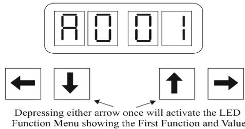
**Figure MMC-343-11: Display Function Menu Activated**
