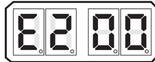
Figure 6-6: Display LED E2 - Servo
