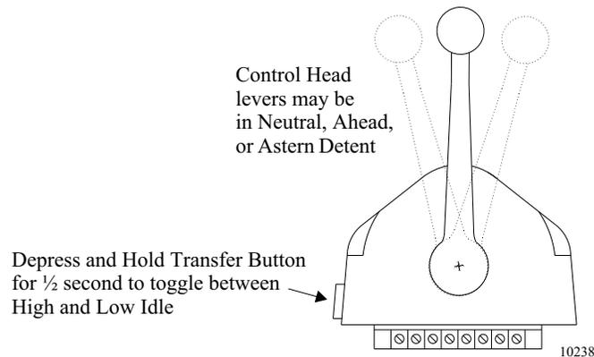
**Figure 2-7: High/Low Idle Mode Selection**
