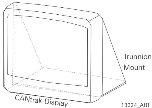
Figure MM70179-15: Trunnion Mounting
