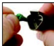
4. Once all contacts are in place, insert wedgelock with arrow pointing toward exterior locking mechanism. The wedgelock will snap into place. Rectangular wedges are not oriented. They may go in either way.
