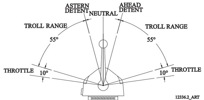
**Figure 5-32: Control Head 45 Degree Troll Range - Type 3**
