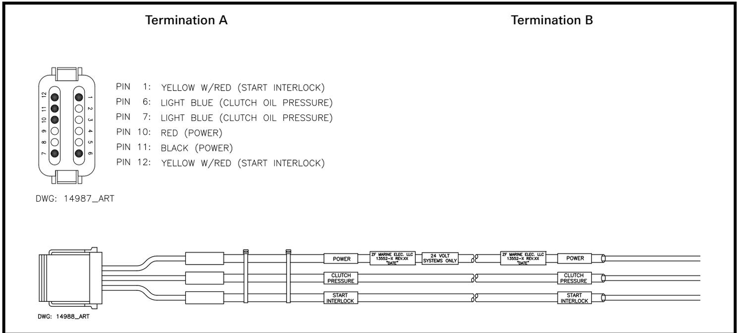
**Table 10-58: Wire Harness - Power, Start Interlock, Clutch Pressure Switch & Alarm (p/n 13631-XX)**
