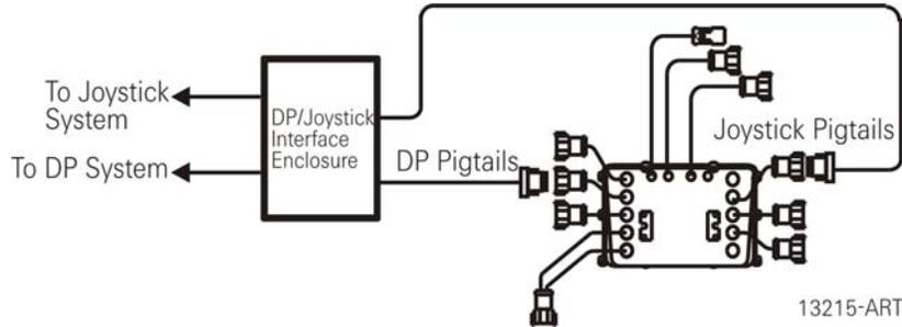
Figure 4-26: DP/JS Enclosure pigtails to Processor Station 5 and Station 4 pigtails
