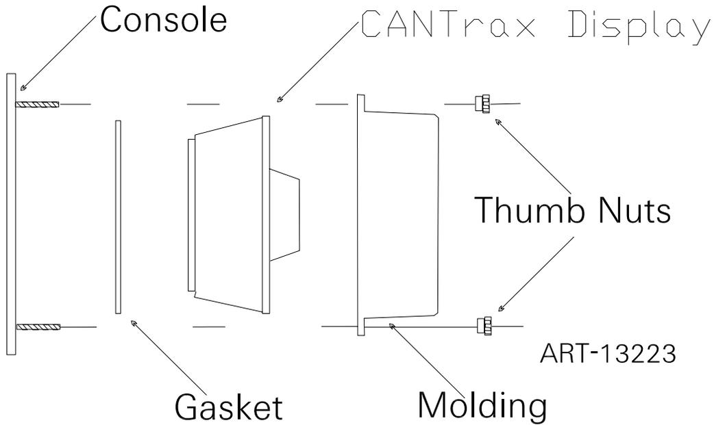
Figure MM70179-14: Behind Console Mounting
