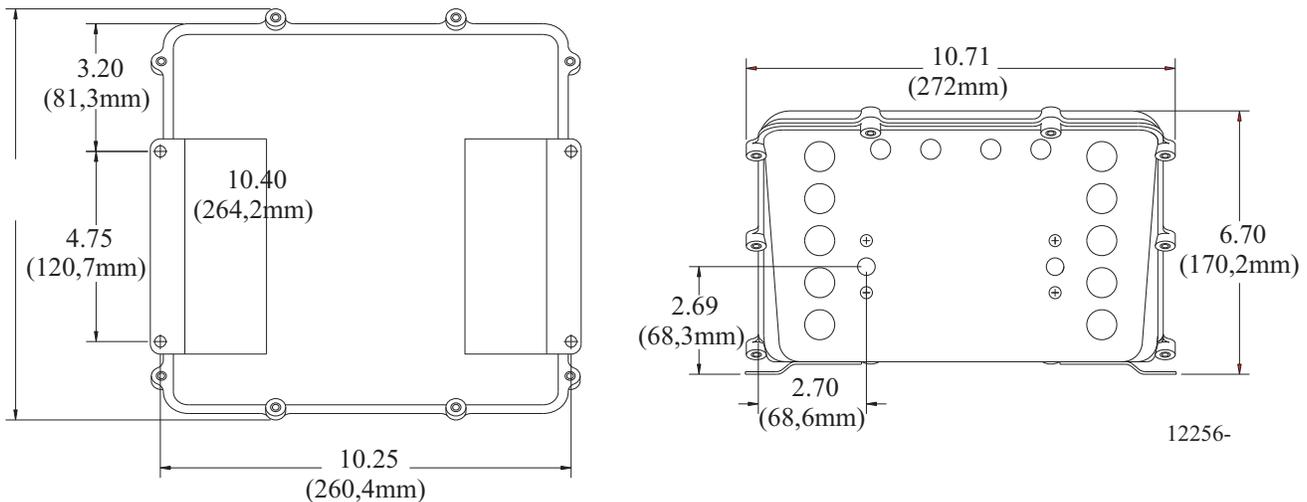
**Figure 3-1: Processor Dimensions**
