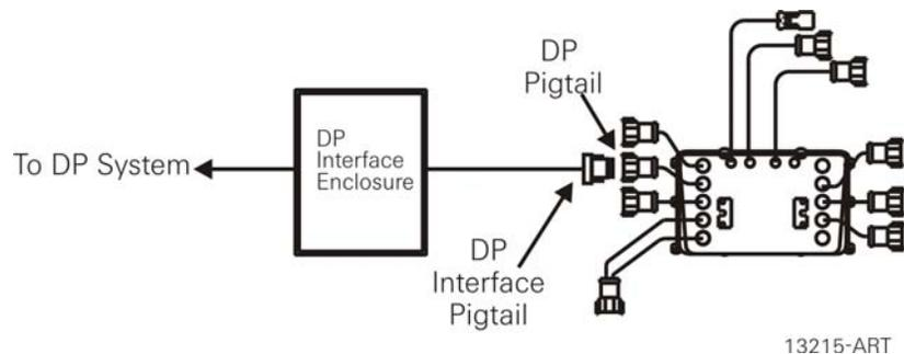
Figure 4-25: Enclosure DP Pigtail to Processor DP Pigtail Connections
