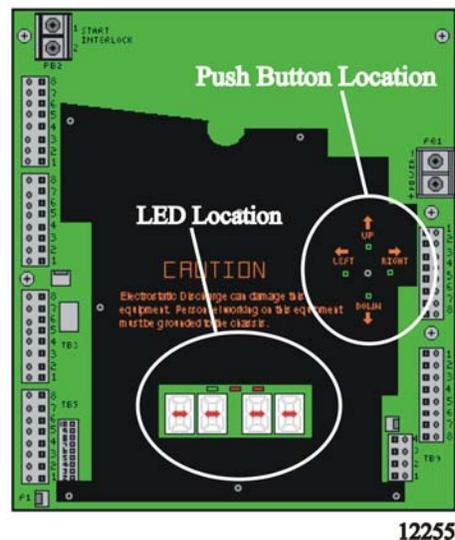
Figure 2-10: Circuit Board Shield Layout
