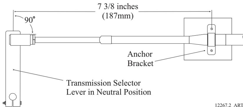
**Figure 4-24: Shift Push-Pull Cable Neutral Connection**
