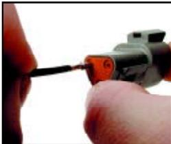
3. Hold the rear seal in place, as removing the contact may displace the seal.
