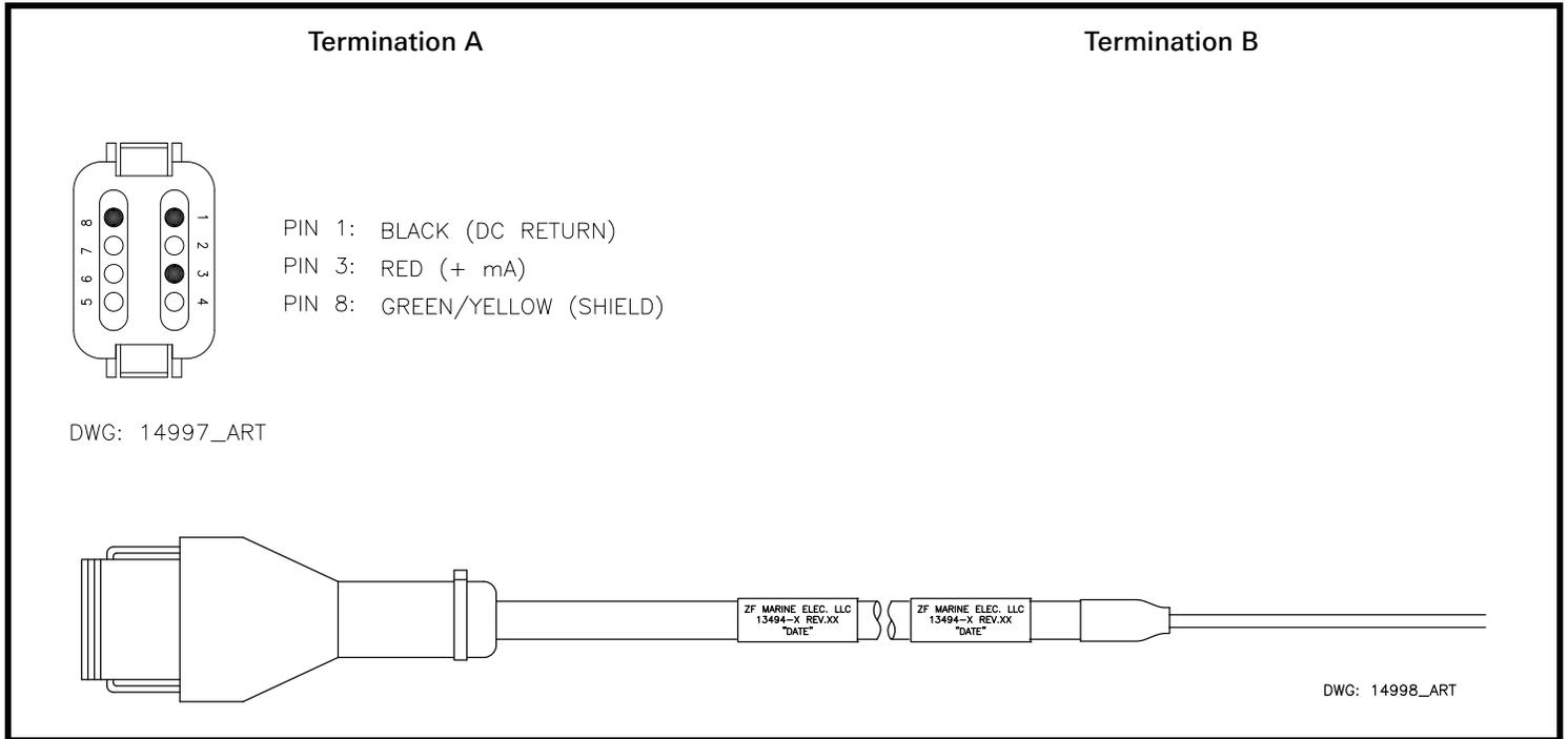
**Table 10-46: Wire Harness - Throttle, Voltage (Cummins Plug), (p/n 13565-XX)**
