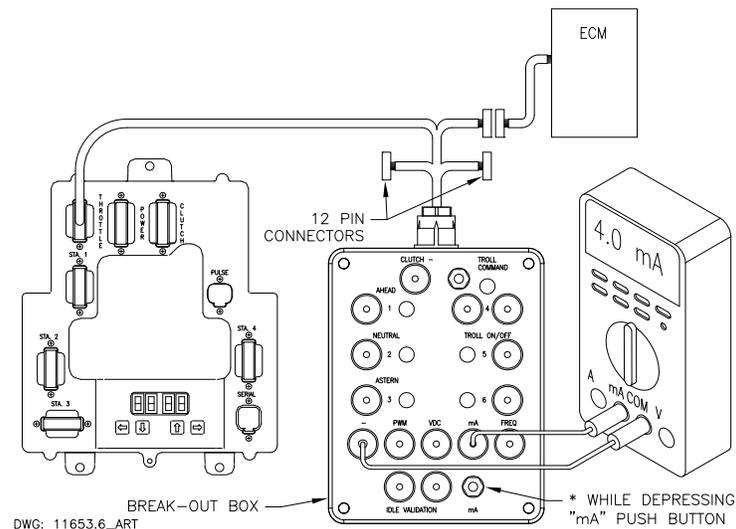
**Figure MM13927-5: Throttle Connection (Current mA)**
