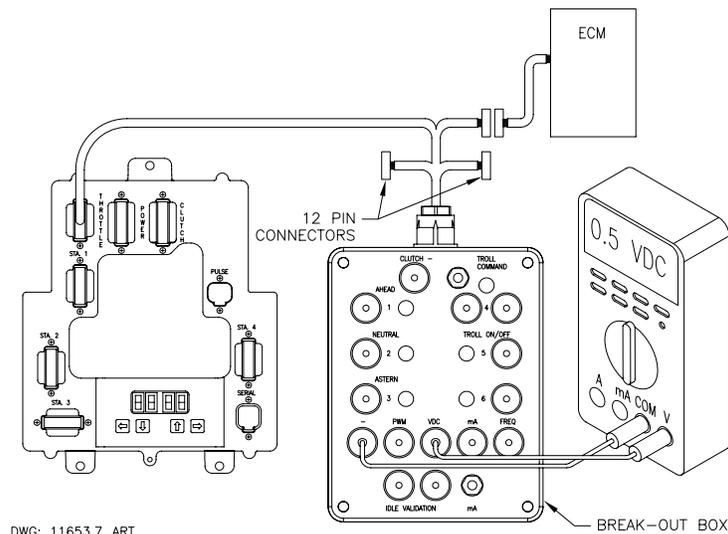
**Figure MM13927-4: Throttle Connection (DC Voltage)**
