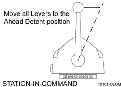
**Figure 2-8: One Lever Operation Mode**
