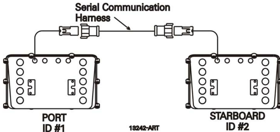
Figure 4-3: Twin Screw Serial Harness Connections
