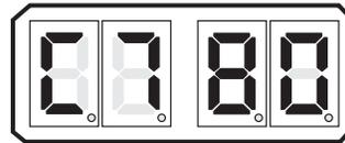
**Figure 5-28: Display LED C7 - Servo**
