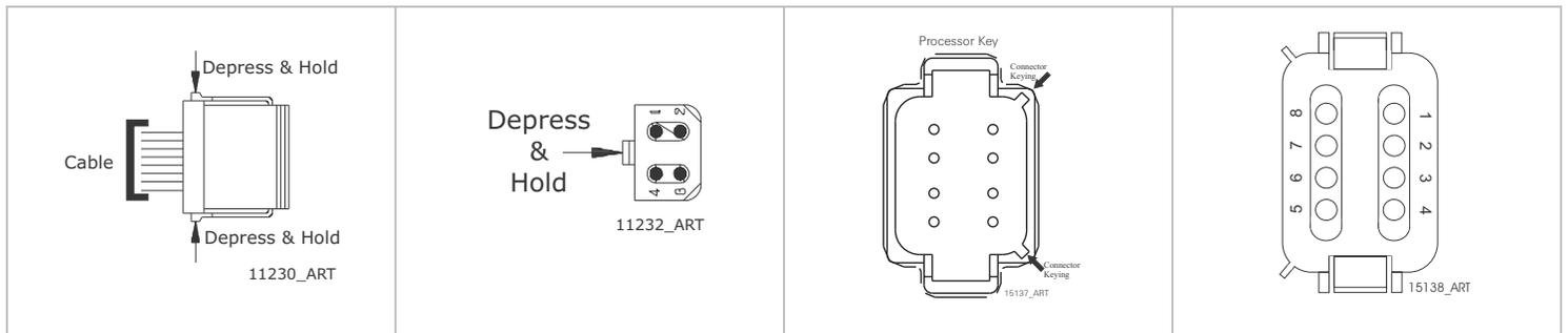
**Figure MMC-343-3: Harness Plug Connectors**
