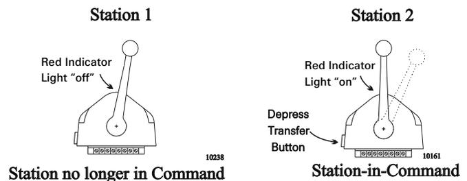
Figure 2-3: Remote Stations Before Transfer of Command
