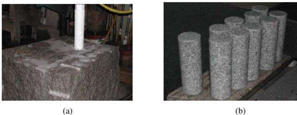
Figure 3.2 Preparation of cylindrical cores for the Material Test Programme: (a) diamond core drilling of intact granite block; (b) cylindrical cores obtained from diamond core drilling
