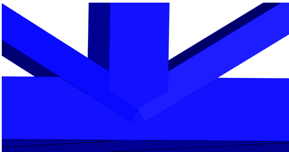
Figure 11-6 Main bracing diagonals oriented along the wind
