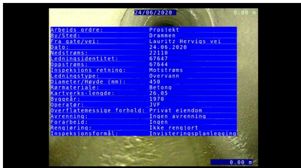
Foto: L67647_67644_22110_24062020_1_1_0_U.JPG, 00:00:00 0m, Start inspeksjon -
