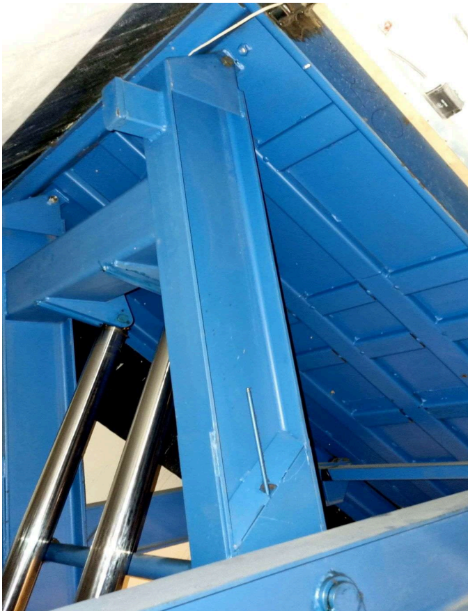
Figur 10 Sylinder, saks, underside plattform - Bakscene
