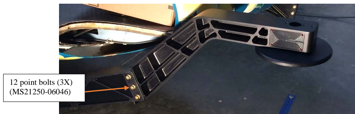
Figure 7 Installation of the Forward Arm for Single Pole Configuration
