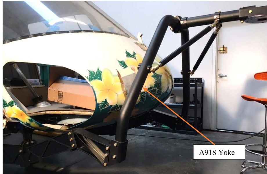
Figure 9 Installation of the A918 Yoke for the Dual Pole Configuration
