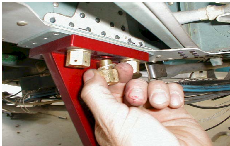
Figure 3 Installation of the Non-Clamping A953 T-Bracket with A700 Nuts
