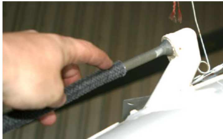
Figure 10 Installation of the Pitot Tube Extension (Tube) onto Pitot Tube
