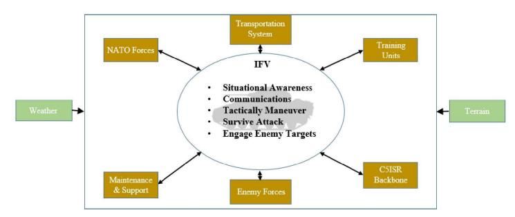
• Figure 1 - The Battalion (Bn) as a system of systems where the Vehicle (one individual) is one system.
