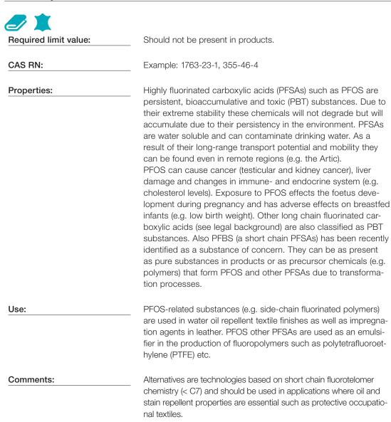
Where oil repellent properties are not essential and just water repellency is required, non-fluorinated chemistries (C0) such as waxes and paraffins but not silicones are requested.
