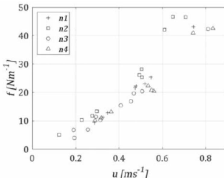
**Figure 20: Average drag force per meter for all kelp ropes as a function of towing velocity (Endresen et al., 2019)**
