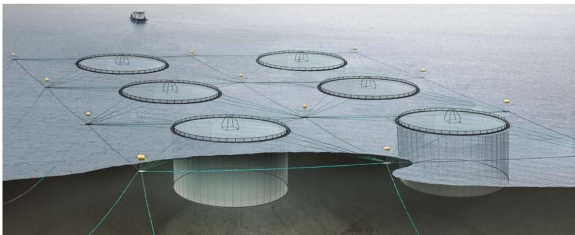
Figure 2: Typical mooring grid configuration used for fish farms (Figure: Akva Group)
