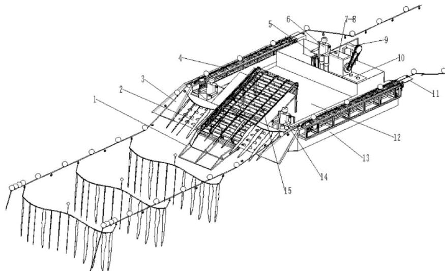
**Figure 11: Mechanized harvesting machine. From (Zhang et al., 2017)**
