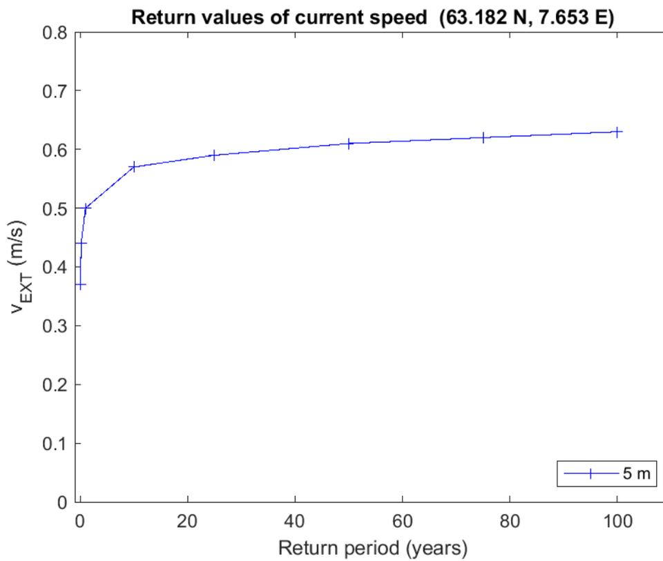
Figure 4 Return values of current speed (depth=5m)
