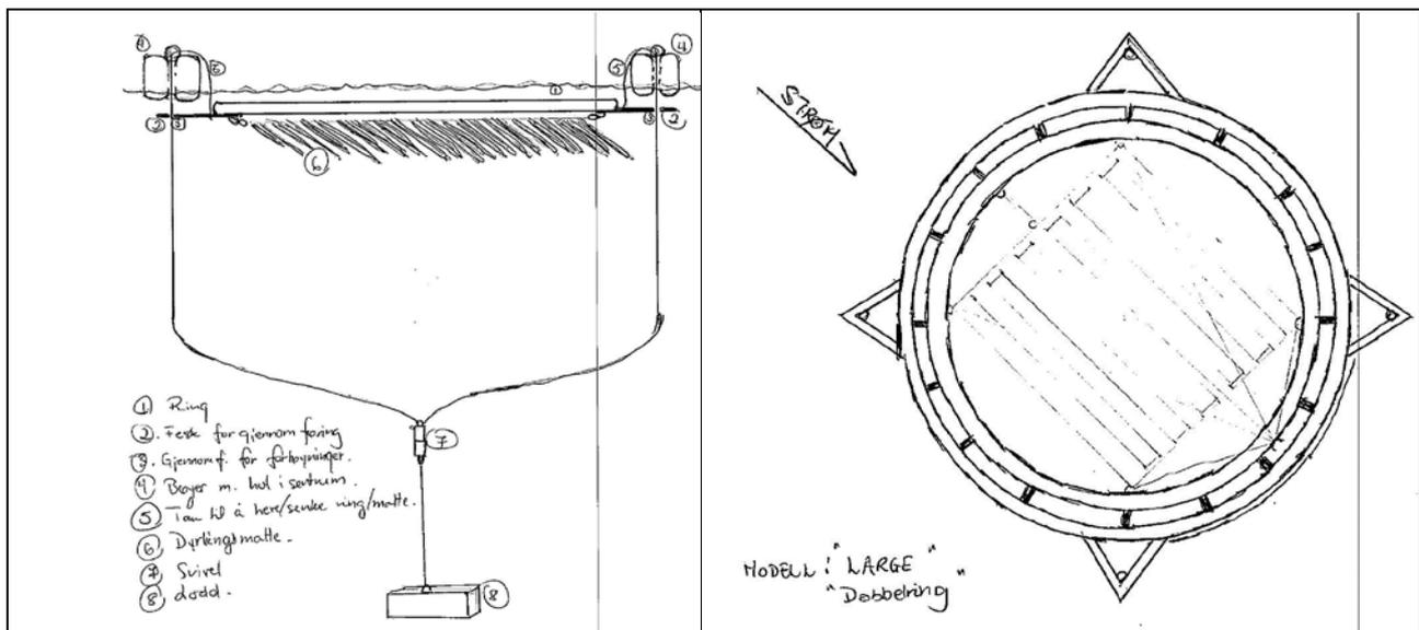
**Figure 17: Sketch of "Proaqua rig" - side view and top view (from Proaqua)**
