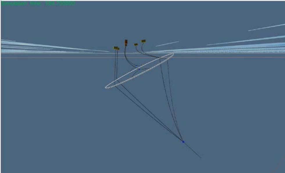
**Figure 18: FhSim - visualisation of results – Proaqua rig in strong current**
