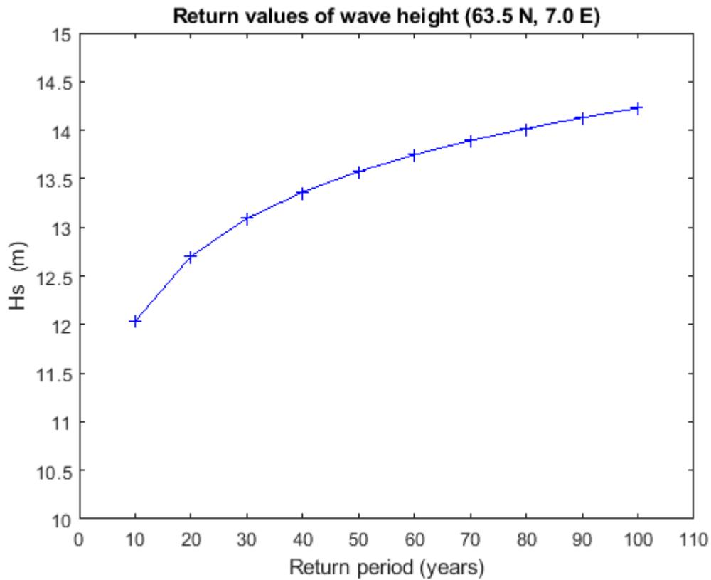
Figure 2 Return values of significant wave height
