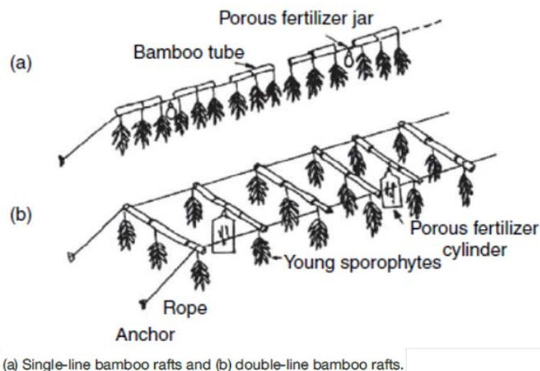
(a) Single-line bamboo rafts and (b) double-line bamboo rafts.
