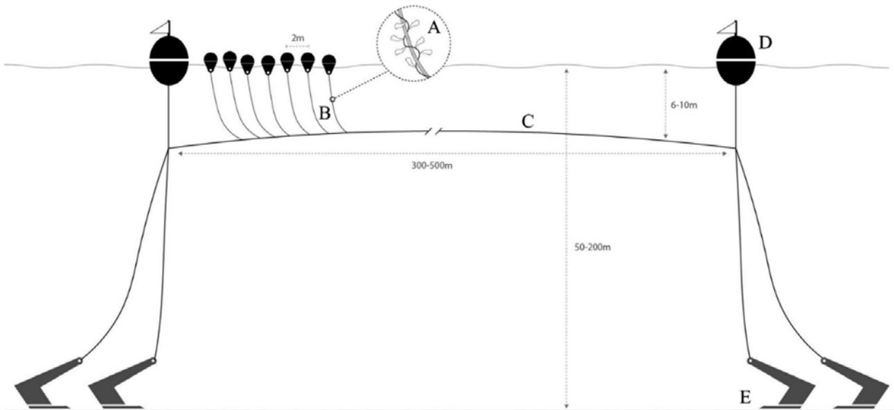
**Figure 5: Schematic drawing of a Macroalgal Cultivation Rig (MACR) by Ocean Rainforest**
