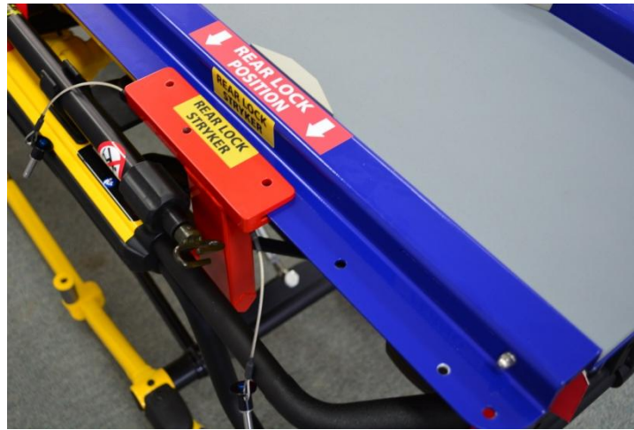
Figure 3: A correctly positioned rear end restraint
