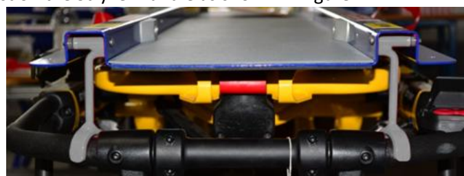
Figure 2: Correct positioning of Stryker handle vertical support brackets
