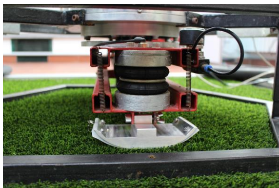
Figure 34: Test foot in position having the load applied
