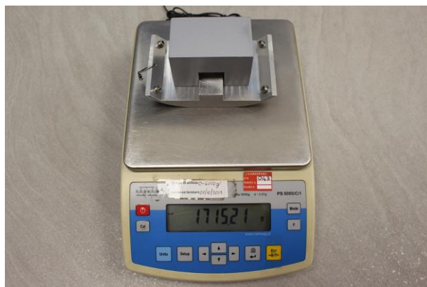
Figure 26: Total mass of the test foot with additional mass
