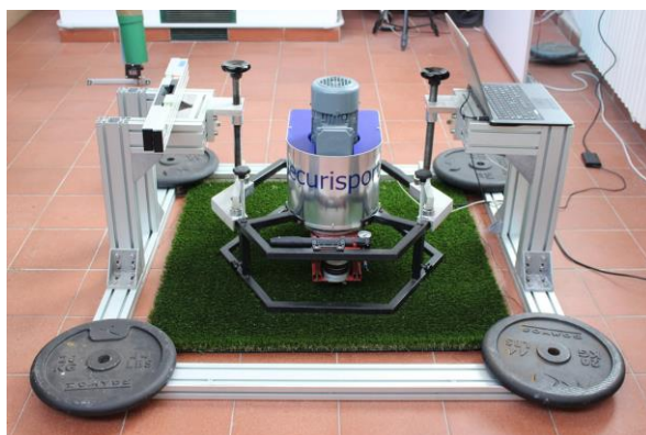
Figure 30: Securisport Sport Surface Tester positioned, stabilized and ready to test
