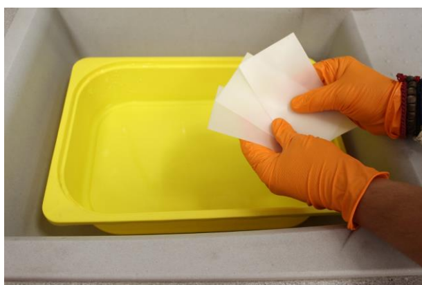
Figure 15: Silicon skin handled with dust free nitrile gloves
