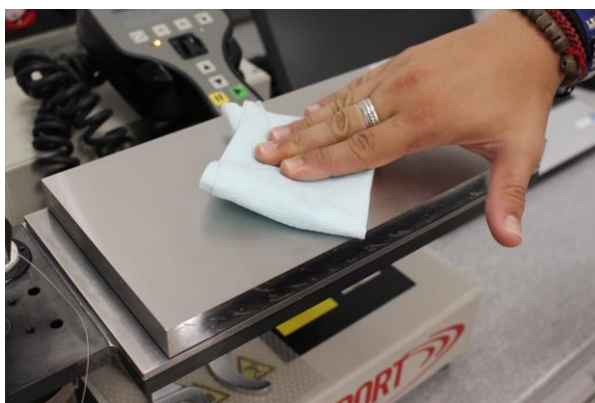
Figure 27: Cleaning of the metal reference plate
