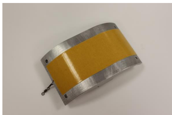
Figure 21: Test foot with double-sided tape
