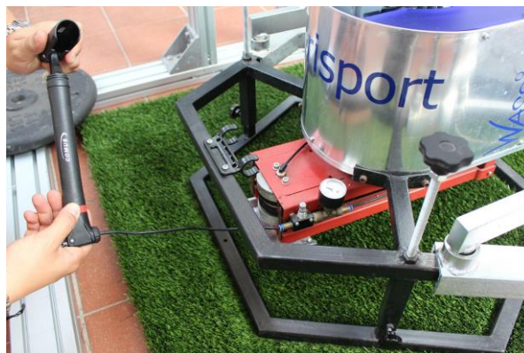
Figure 33: Applying pressure to obtain 100\text{N} \pm 10\text{N}
