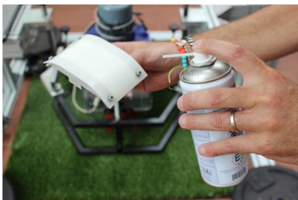
Figure 35: Cleaning with DRY compressed air
