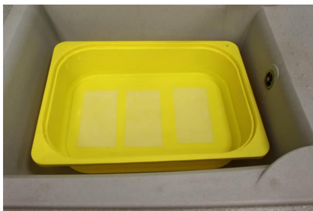
Figure 16: Skins immersed in water with smooth surface upward
