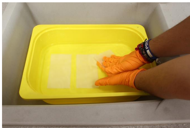
Figure 17: Cleaning the silicon skins
