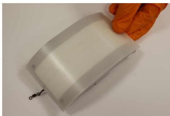
Figure 22: Test foot with the silicon skin taped
