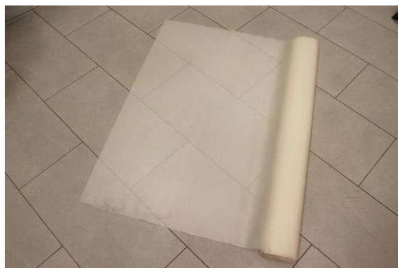
Figure 11: Roll of silicon skin with smooth side upward
