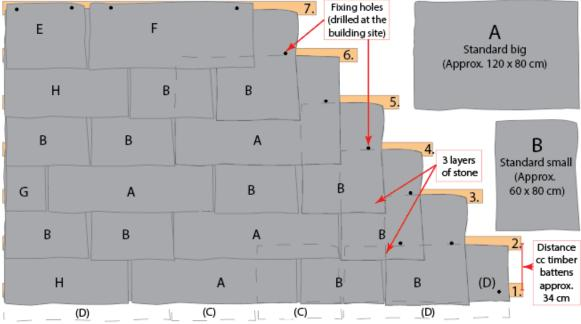
Roofing system made from a system of 2 different standard stones A and B (Buildt on repetitions of A = 1 pcs 120x80cm and B = 2 pcs 60x80cm)
