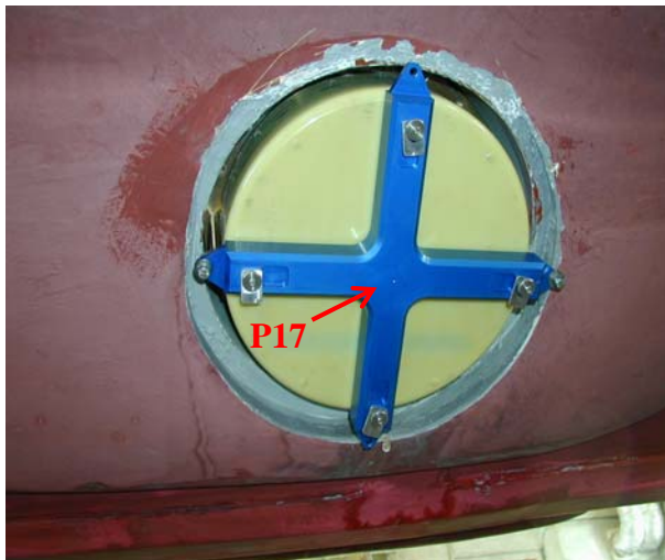
Figure 10 Benchmark 17 – Port centre laser tool
