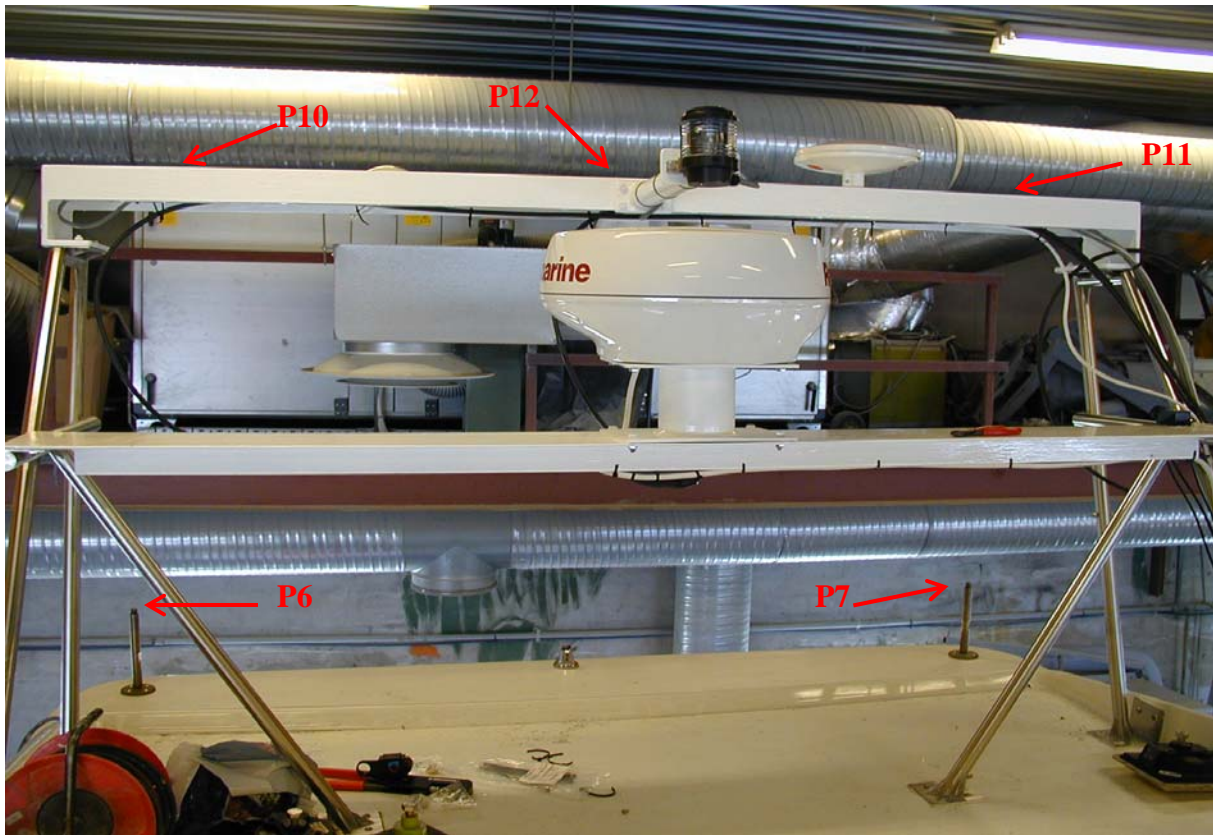
Figure 6 Benchmark P6, P7, P10, P11 and P12. P6 (starboard) and P7 (port) – GPS antenna mount on rear wheelhouse roof. P10 (starboard) and P11 (port) are at the top of the centre of the drilled hole of the Seapath bar. P12 is for the Abspos antenna.
