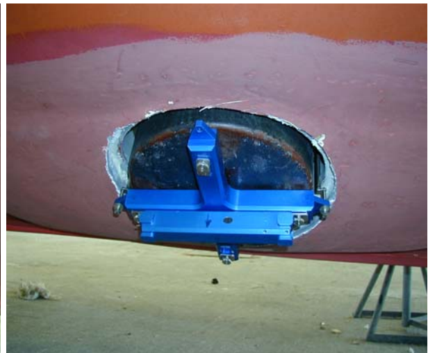
Figure 11 Starboard transducer with laser measuring tool mounted on it
