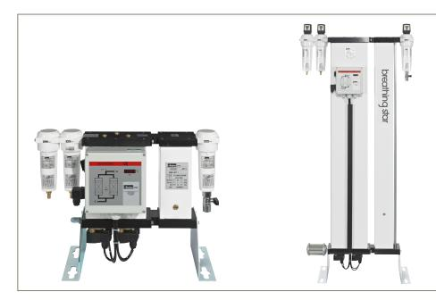
Dry compressed air subsequently enters the integral purification and catalytic stage where oil-vapour, odours, gaseous vapours and traces of carbon-monoxide are reliably removed. Finally, the clean, treated air exits via the validated GL after-filter into the downstream compressed air network.
